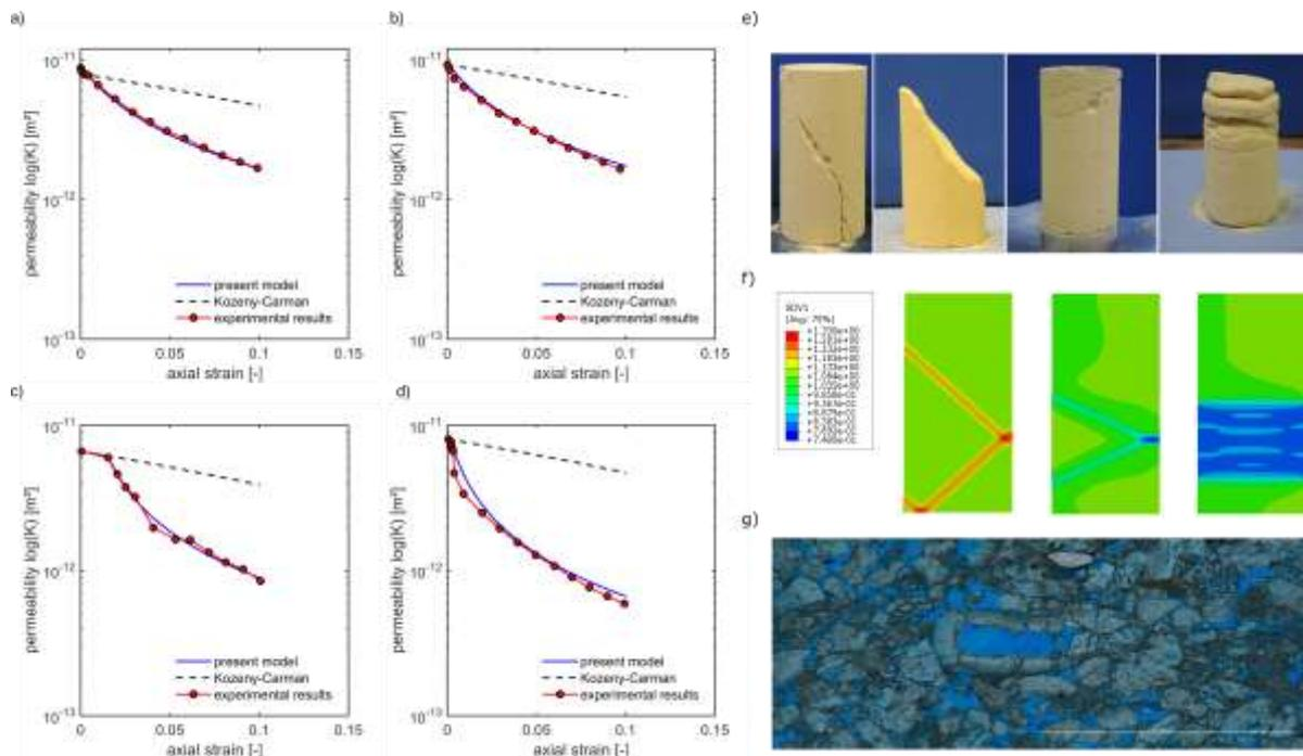
**Figure 1** a-d: results of the analytical model based on the Kozeny-Carman equation and experimental results from drained triaxial tests with different confining pressures: permeability in axial direction plotted in logarithmic scale against axial strain. e) samples after triaxial tests under dry conditions at different confining pressures, f) numerical results of biaxial test with different confining pressures, g) thin section of the compacted rock
