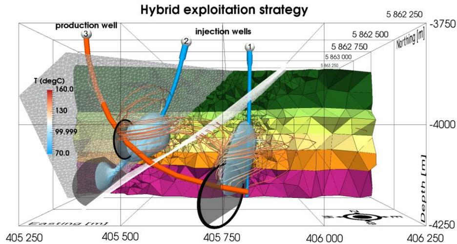
**Figure 1:** Example of results obtained from a simulation of the Groß Schönebeck geothermal reservoirs illustrating the evolution of the breakthrough temperature together with flowlines after approximately 30 years.
