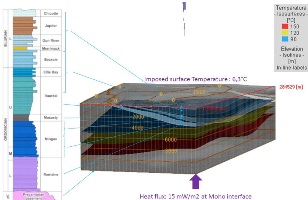
Illustration 1: Thermal model for Anticosti basin (Feflow) based on a geological model (Gocad)
