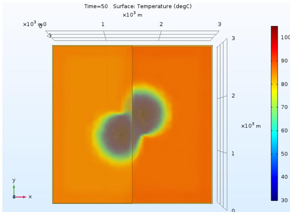
**Figure 1. Top view of domain temperature after 50 years of production for one parameter combination**
